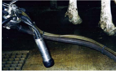
Keeping hoses together allows for better alignment
