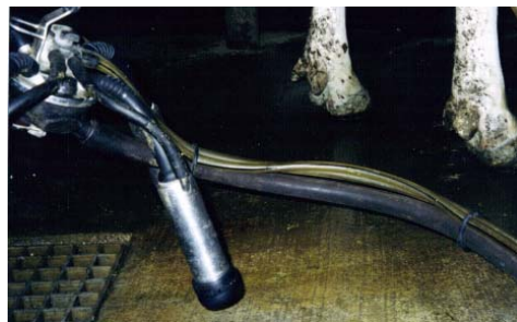
Keeping hoses together allows for better alignment
